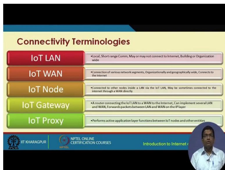
So, in terms of connectivity, we are talking about concepts called Unique Building Blocks, such as the LAN IoT, WAN IoT, Node IoT, Gateway IoT, Proxy and so on and so forth. So, all most analogist to what we have as different components of the internet, the capital I internet means the internet of computers analogously. We are also going to
