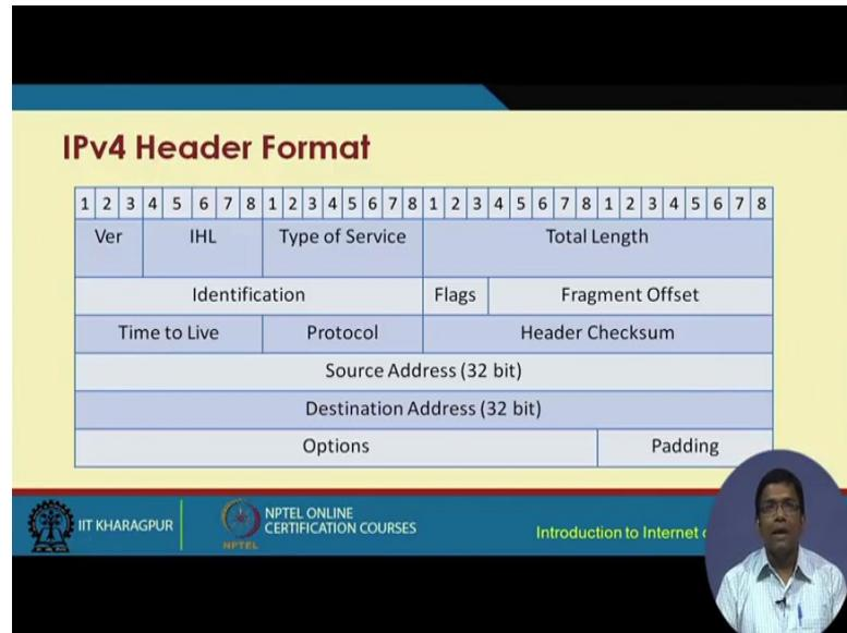
So, here are few other points of comparison which I am not going to go through and here is the IPv4 header format.
