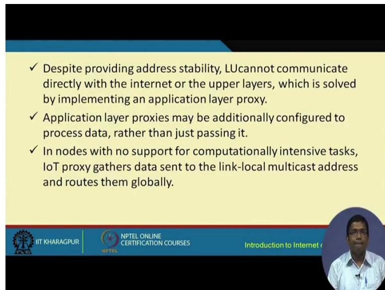
✓ Despite providing address stability, LU cannot communicate directly with the internet or the upper layers, which is solved by implementing an application layer proxy.
