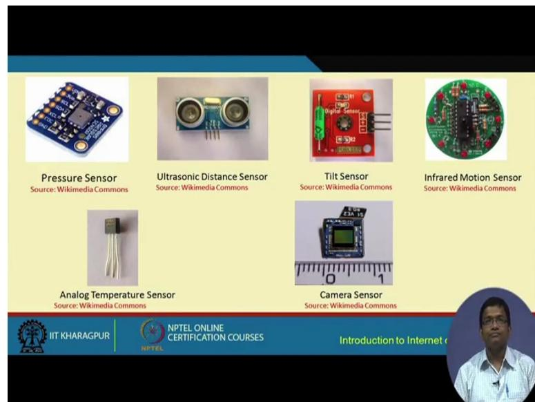
So, I had already in at the outset of this lecture, I had shown you some real physical sensors. Here are some other pi pictures of few other sensors, here is a pressure sensor, here is an ultrasonic distance sensor, tilt sensor infrared motion sensor, camera sensor, analog temperature sensor. So, analogs in temperature sensor, it has you know in
