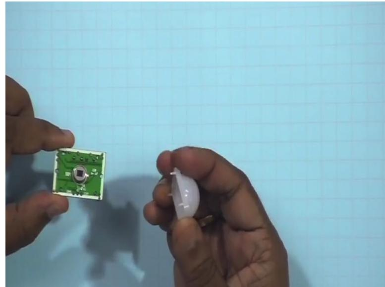
So, here are few real sensors and this is a sensor that is used for obstacle detection. This is a PIR sensor passive infrared sensors. So, this passive infrared sensor here can be used for detecting if there is any obstacle. So, this is an example of a PIR or obstacle based sensor.
