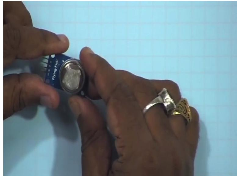
Finally, I would like to show you another sensor which is the temperature and humidity sensor. This is actually, this measures both of these together this particular sensor.
