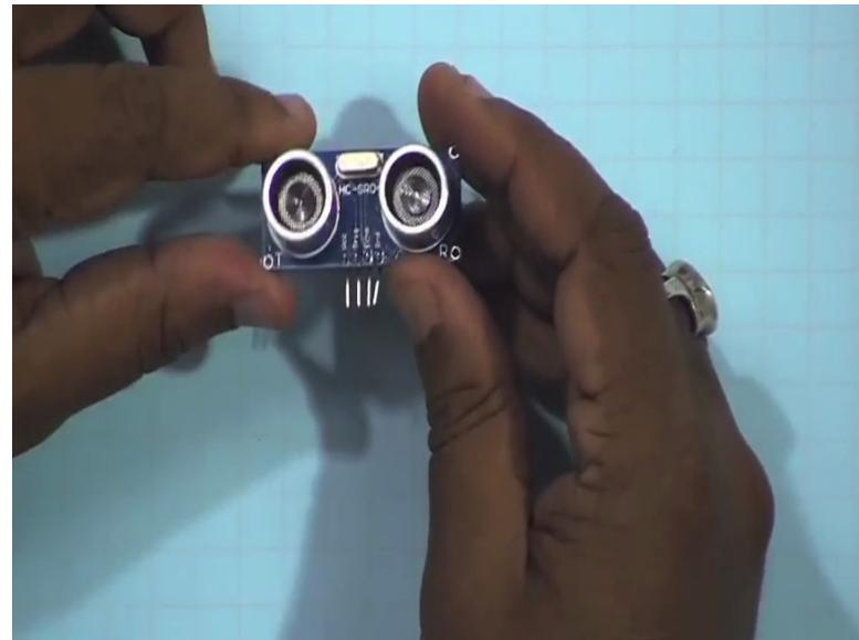
Then, we have another sensor this is the ultrasonic sensor. This basically detects that how far that obstacle is. This is another sensor. So, here as you can see that there are like two eyes kind of things. So, what happens is these ultrasonic sensors may send
