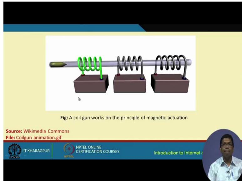
Fig: A coil gun works on the principle of magnetic actuation
