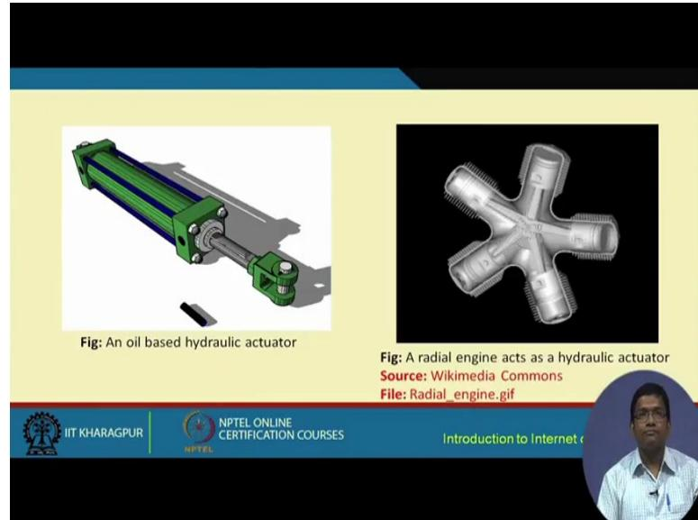
On the left hand side, we see an example of an hydraulic actuator which is based on the use of oil. So, in this particular cylinder, oil will be there and then, when you put, when you apply pressure on it, it is going to give an output based on which there can be some linear motion or some oscillatory motion or rotatory motion or whatever that can be performed.
