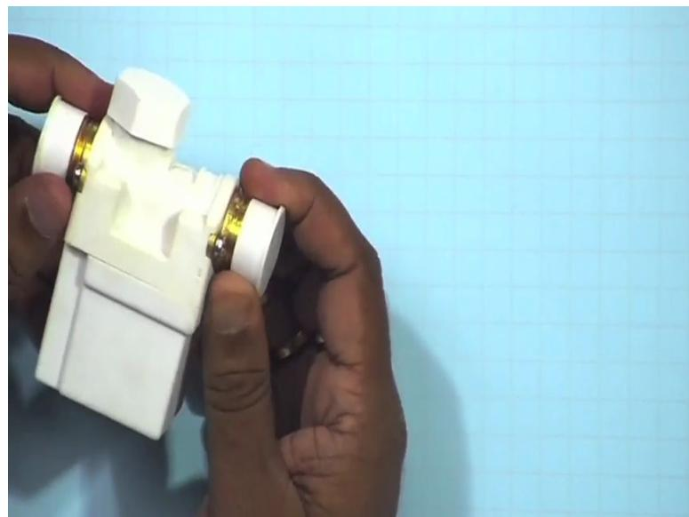
There is another one which is the solenoid valve and this basically can help in controlling the flow of liquid. So, you have an input; you have an output. So, we have an input, we have an output and the solenoid valve if we open it, so what we can see over here is what is inside. So, you know water can flow in and depending on the conditions, this valve is going to either allow the water to flow out or it is going to stop. It is not going to allow.
