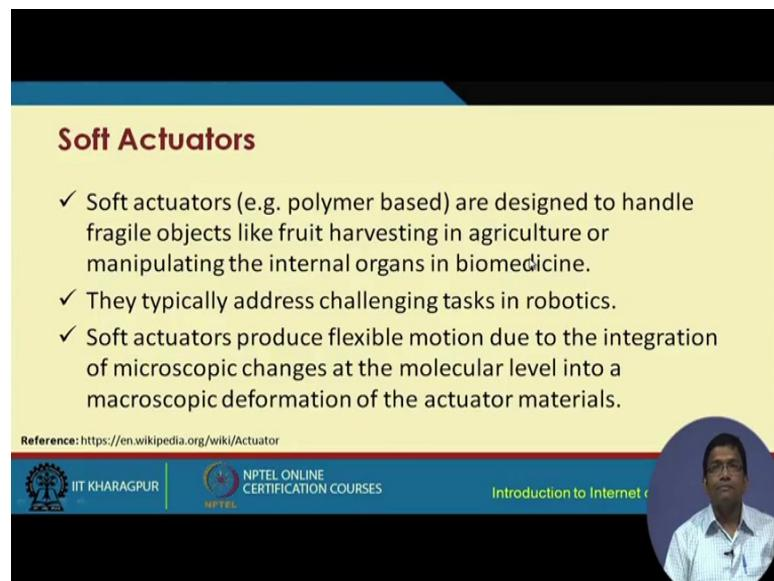
So, as this thing moves in this manner, so this gives this one a mechanical motion, a rotatory motion. There are different soft actuators which are actually polymer based and the design to handle fragile objects like fruit harvesting in agriculture or in biomedicine, handling internal organs of human beings and typically these are used in robotics. So, soft actuators are also quite popular.
