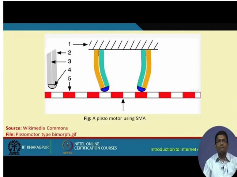
So, this is how it works. So, this is an example of an SMA based piezo motor. So, as you can see over here, these are the different steps in which it works. So, these are two metal strips and when you know when the energy is passed through it, they bend and when they bend, they basically move this red and white strip mechanically. So, this basically acts as an actuator.
