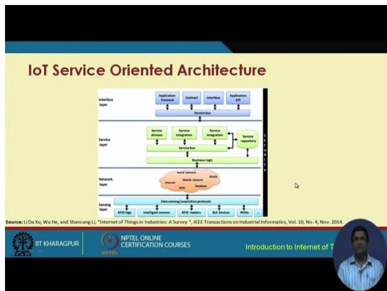
Now, let us look at the service orientation, the service oriented architecture of IoT. So, in the IoT if here what we have at these different layers, the sensing layer, the network layer, the service layer and the interface layer.
