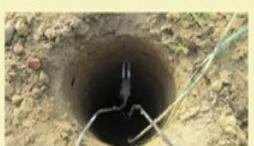
Fig 5: EC-05 soil moisture sensor
