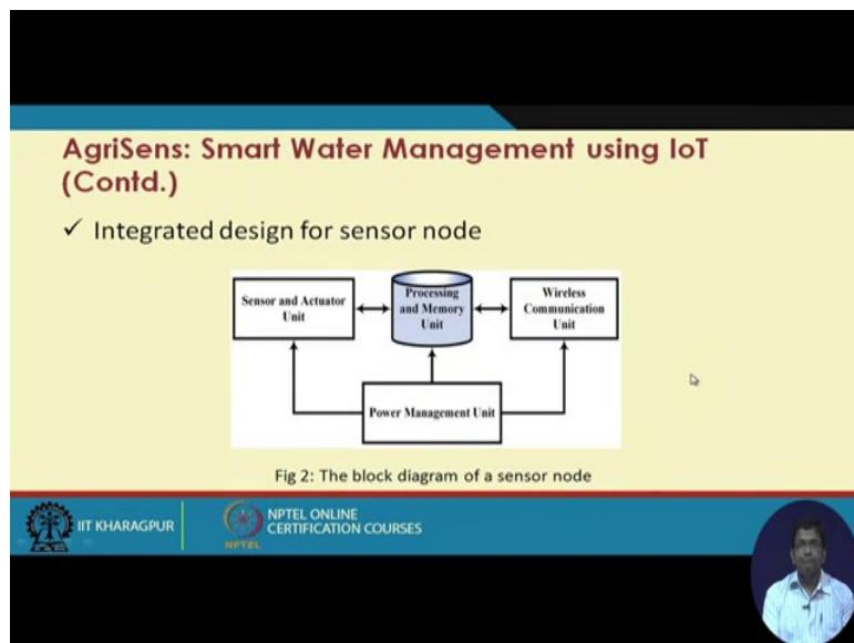
So, this is the overall design of the sensor node. So, here basically what we have is apart from the sensors and actuators we have a processing unit and the memory unit we have wireless communication unit and we have the power management unit.
