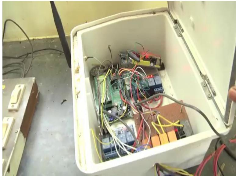
So, as I told you that we are actually following cluster based architecture for the sensor deployment so here what we have is a cluster head this cluster head has support for both Zigbee communication which is happening through this particular node and there is also
